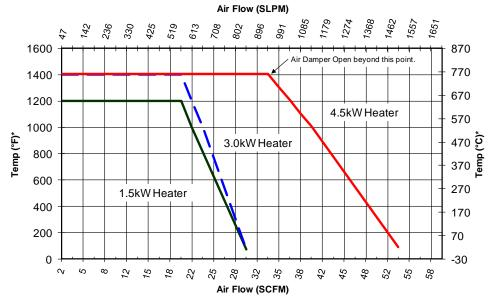
\* Air Tempeature as measured by internal "K" thermocouple
