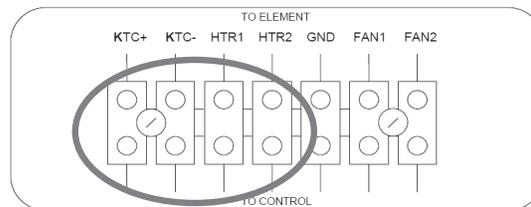
5. Remove the old element, pulling the KTC and HTR wires through the plastic support tower.
