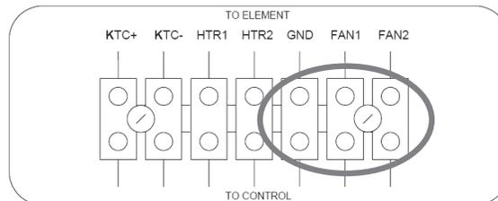
5. Remove the blower, GND, FAN1, FAN2 wires through the plastic support tower.
