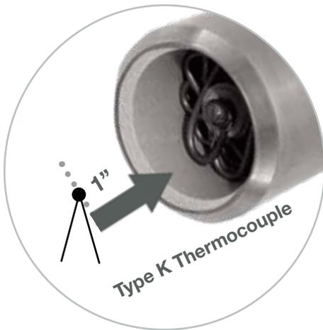
TC placement is very important. The exposed TC junction should be no further than 1" from the Serpentine element (Left).
