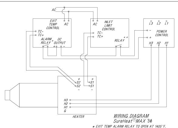
\*\* INLET LIMIT RELAY TO OPEN AT 300°F.
