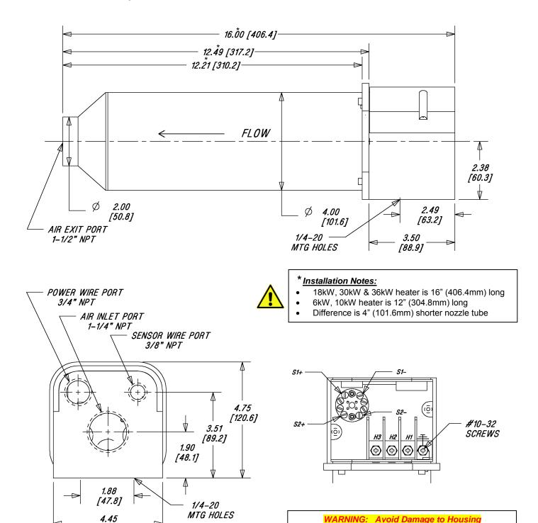
3/8" NPT (Sensor): 4 ft-lb 3/4" NPT (Power): 25 ft-lb 1-1/4" NPT (Air): 7 ft-lb (Excessive force will crack housing and void warranty)
