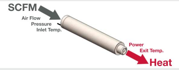
To calculate power requirements; use the above example and desired exit temperature of 800°F.
