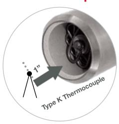
TC placement is very important. The exposed TC junction should be no further than 1" from the Serpentine element (Left).
